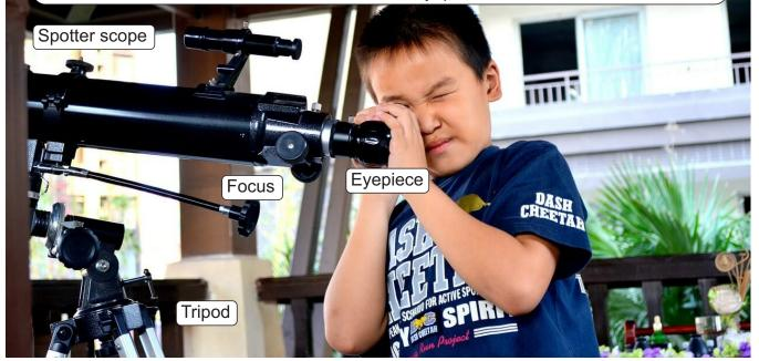
**The tripod** - set it up on stable ground first before attaching telescope - it does not have to be perfectly level. Do not lose/unscrew any pieces - just loosen and tighten as required. Do not knock it over in the dark.
